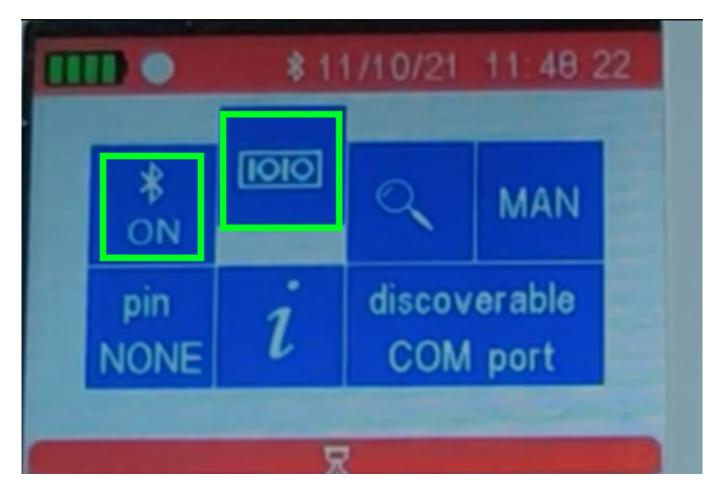
For iOS mobile phones, make sure to have the apple symbol selected and not the SPP as per the picture above to correctly connect your iOS mobile with the OMNI MAX Datamars scanner.
