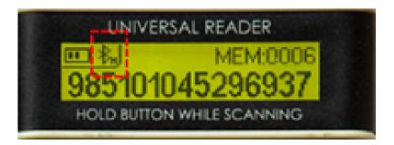
Please note: if the Bluetooth symbol is not flashing, it might mean that the GPR+ scanner is already connected to another device.
